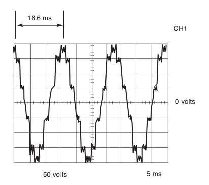
This is the typical auxiliary output voltage generated from a properly operating machine. Note that each vertical division represents 50 volts and that each horizontal division represents 5 milliseconds in time.
