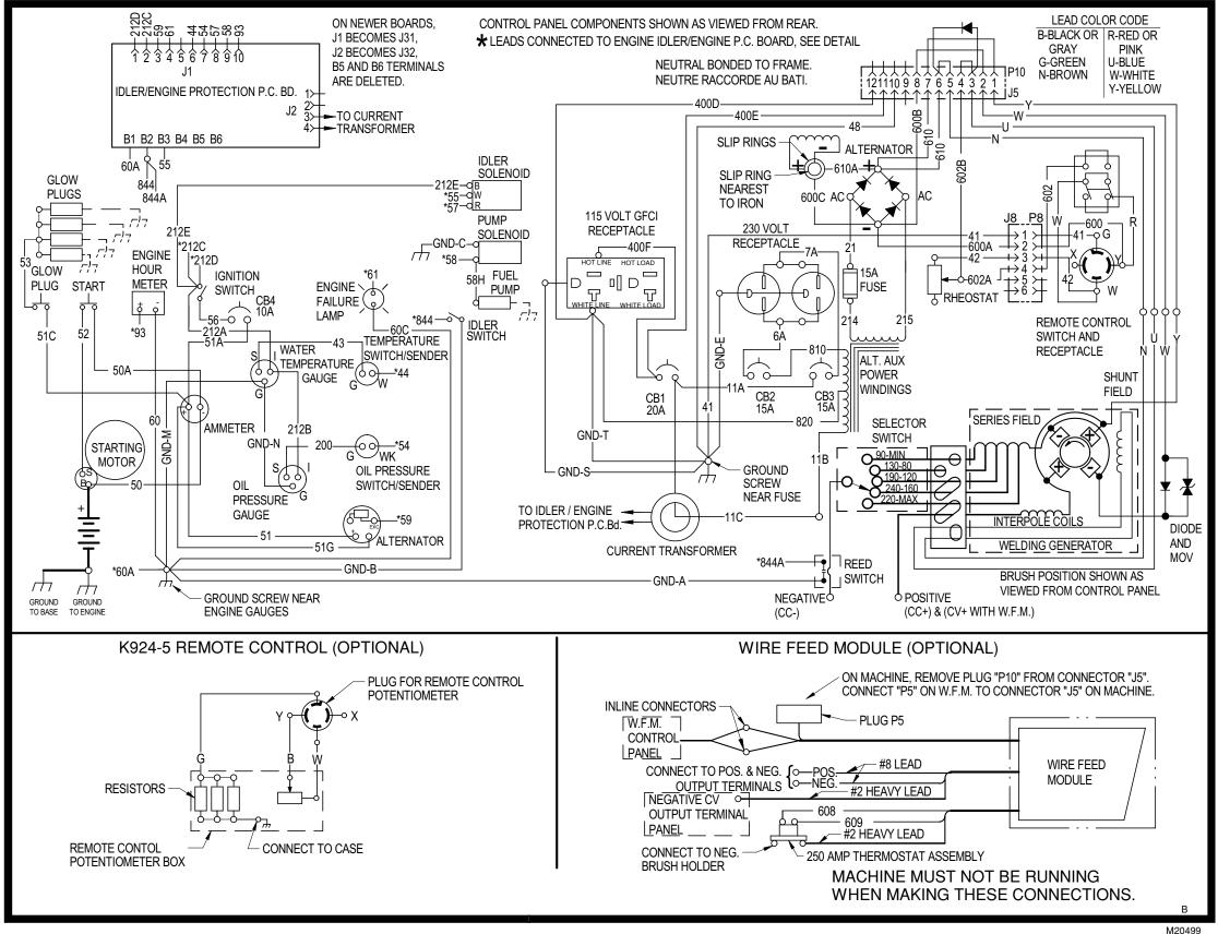
NOTE: This diagram is for reference only. It may not be accurate for all machines covered by this manual. The wiring diagram specific to your code is pasted inside one of the enclosure panels of your machine.
