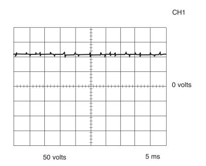
This is the typical DC output voltage generated from a properly operating machine. Note that each vertical division represents 50 volts and that each horizontal division represents 5 milliseconds in time.
