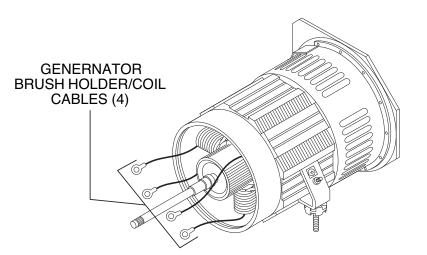
15. With the 1/2" wrench, disconnect and clear the four heavy cables from the generator brush holders to the coils in the generator frame. It is not necessary to remove the brush holder jumper cables. See Figure F.10. Label leads and positions for re-assembly.
