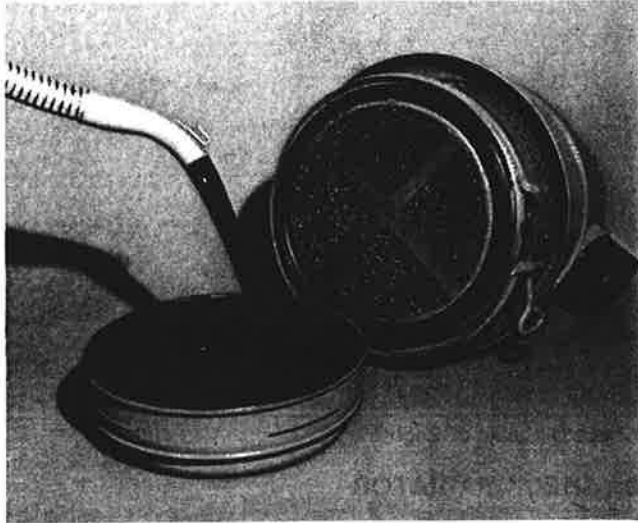
Sectional View of Oil Bath Cleaner
